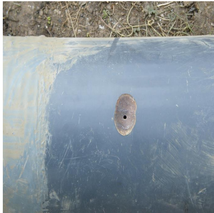
Figure 11 A.C. corrosion defect current density 450 to 600 Am -2 8" intermediate pressure < 7bar gas main
